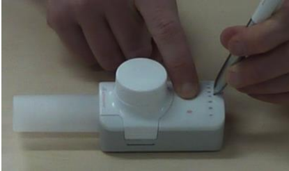
Figure 7: Press the “ON/OFF” key and the “inhalation time” key simultaneously using a pen to press the “inhalation time” key.
